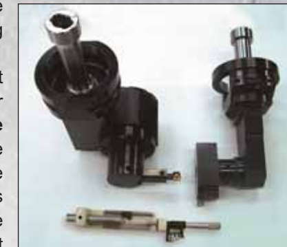
Rottler right angle line boring tools
